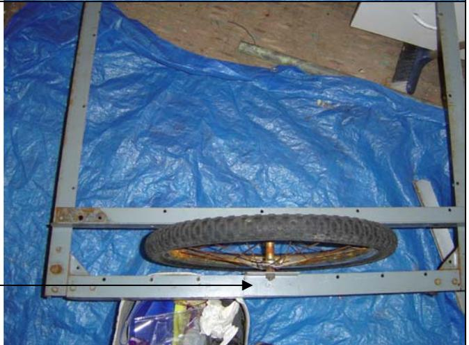
10. Bolt the ends of the long inside wheel support to the underside of the bed frame. Again ensure the wheel and wheel support is as straight as possible. Use two 6mm x 20mm bolts.
