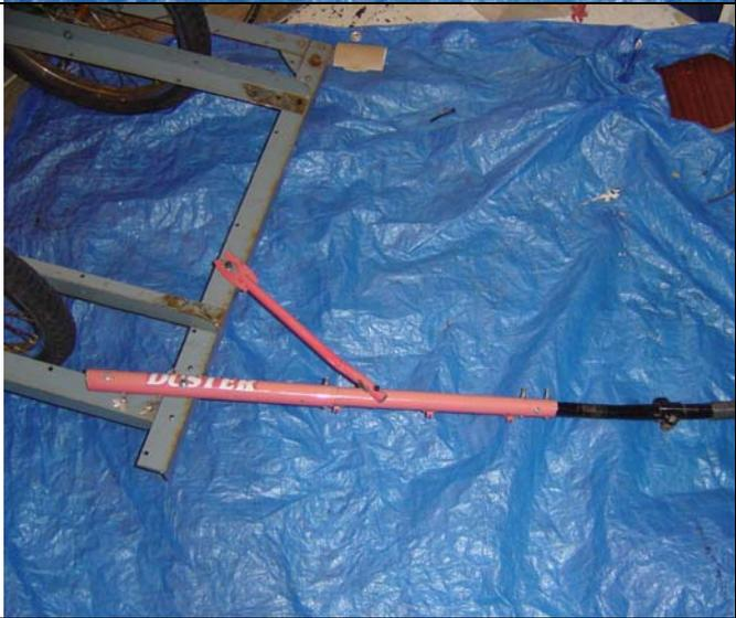
27. If there are not already holes where the springs were removed, drill some holes for hooking bungy chords into.
