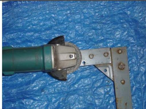
3. Mark and cut two lengths of angle iron off the two long edges of the bed that are the same length as the width of the bed (typically 900mm). These are the *inside wheel supports*.
