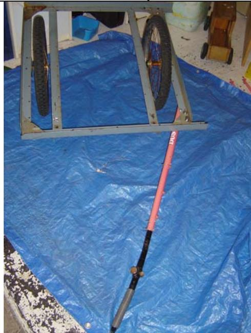
25. Cut a piece of pipe off the bike to use for a brace. One of the rear wheel supports has a nice bend that helps line it up with the bottom of the tow bar which is lower than the frame of the trailer.
