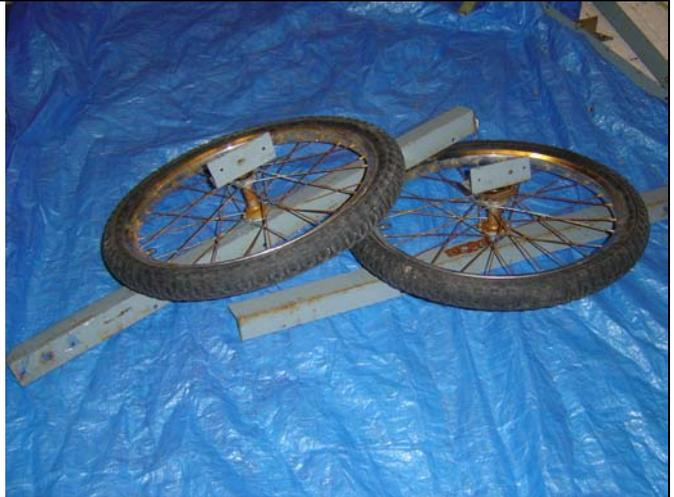
9. Support the main frame of the trailer on blocks. Drill holes and bolt one of the 100mm outside wheel supports to underside of the right hand edge of the bed frame in the centre of the frame, ensuring the wheel is as straight as possible. Use two 6mm x 20mm bolts.
