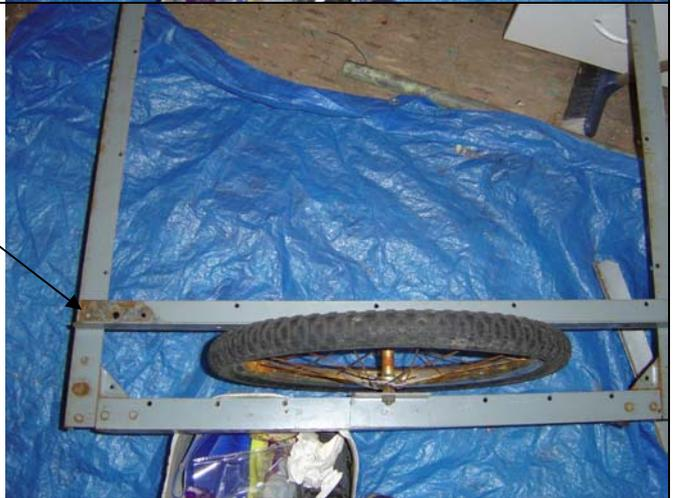
11. Get your bins and place them against the long wheel support. Place the other long inside wheel support (with wheel fitted) against the other edge of the bin and mark it's position such that the bin is a snug fit between the two wheel supports.
