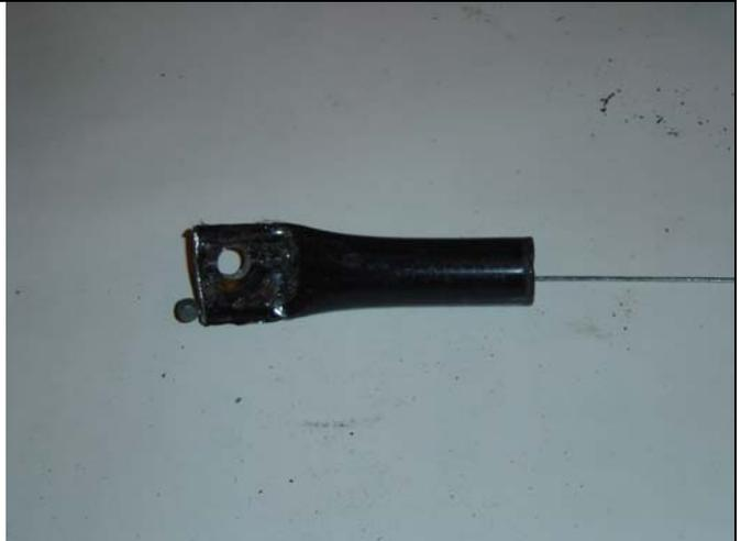
19. Put the hitch together with the brake cable through the centre of the trampoline spring and through a hole drilled in the end of the tow bar a few cm beyond where the spring will end up.
