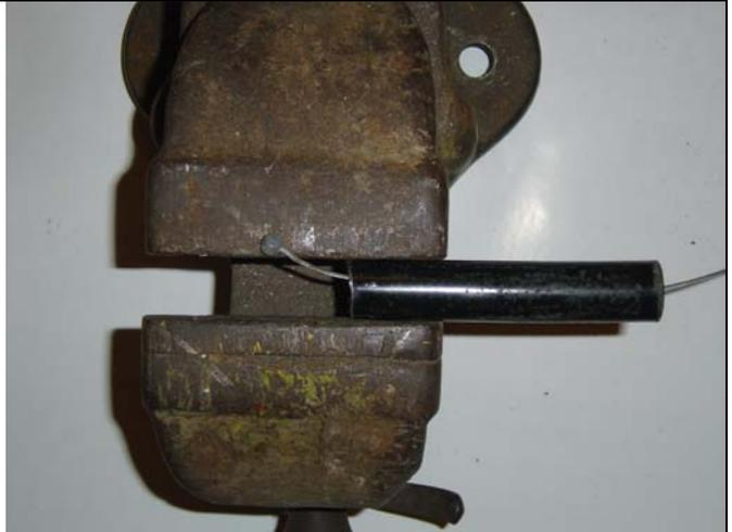
17. Bend the squashed pipe with a hammer to about 20 degrees. Don't over-bend it or it may crack after a bit of use. This is where the trailer will bolt on to the rear wheel of the bike. You could avoid this step by buying one of my pre-made hitch bases for \$15, which is stronger and gives a better angle.
