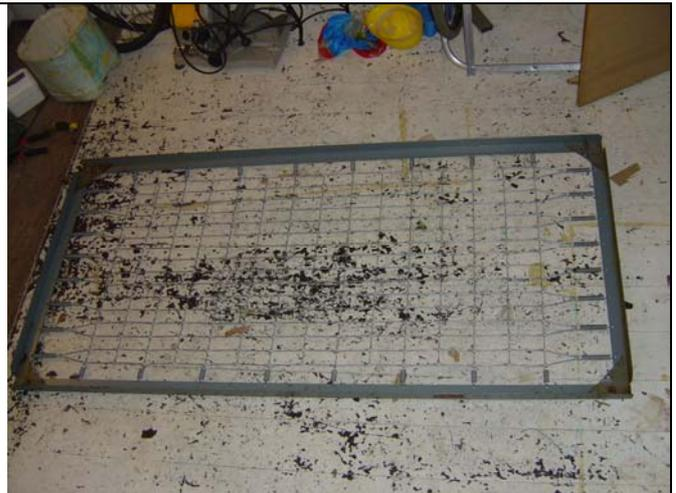
2. Remove the right hand end of bed frame with a spanner, or if its welded, use a hacksaw or angle grinder with metal cutting blade.
