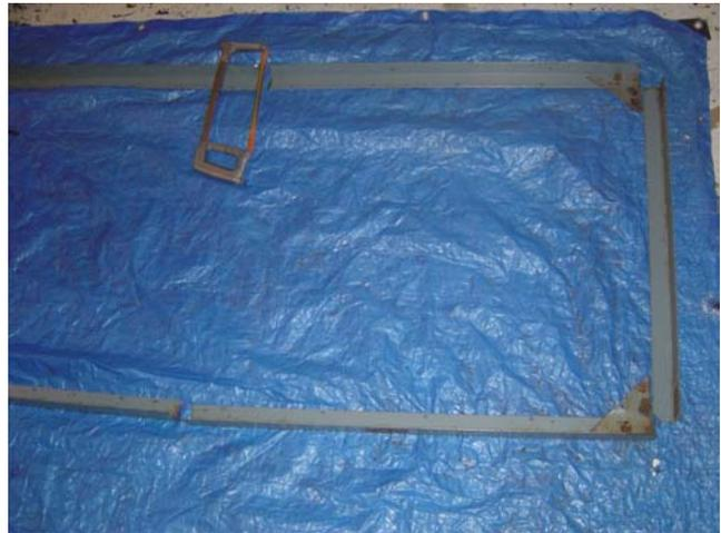
4. Cut a further two 100mm lengths off the two long edges of the bed. These are the *outside wheel supports*.
