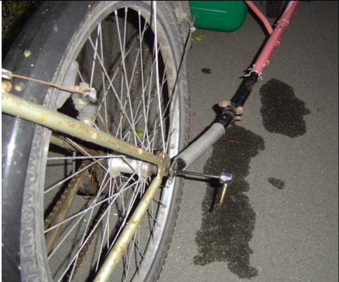
30. Check what happens on a hard right turn. Make sure the tow bar hits the rubber of the wheel and nothing touches the spokes (unless you want expensive wheels repairs).
