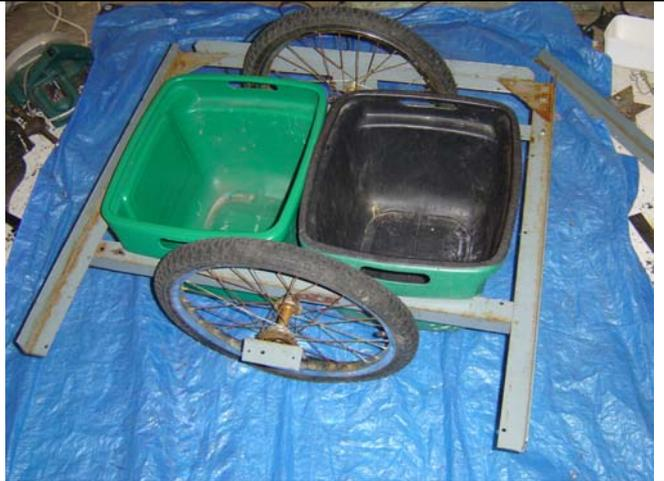
12. Drill and bolt the second long wheel support into place. Again ensure the wheel and wheel support is as straight as possible. Use two 6mm x 20mm bolts.
