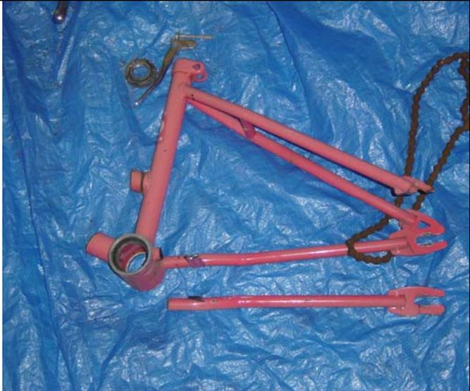
26. Bolt the brace between the frame and the tow bar (underside of the trailer).
