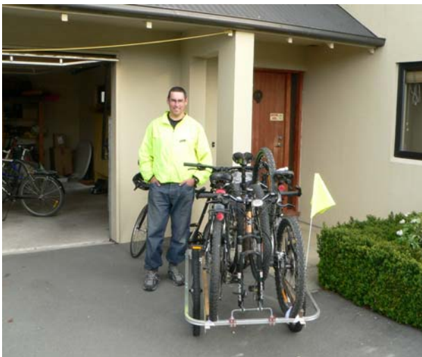
Three bikes being collected by bike trailer using a bent threaded rod bracket to secure the front forks.
