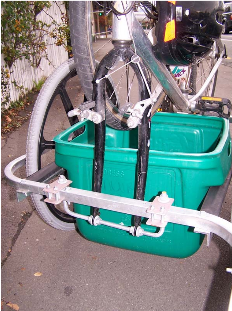
Front fork attachment bracket, Home made from 10mm threaded rod.
