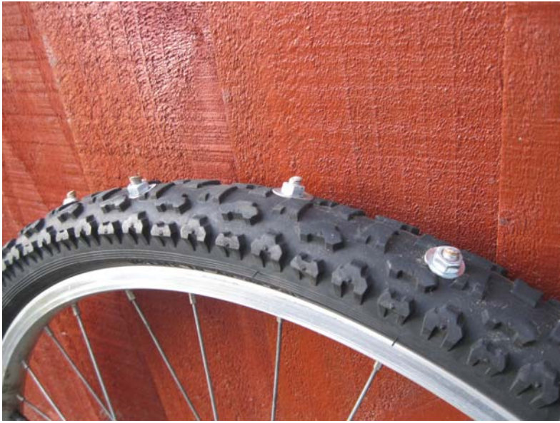
Snow tyre with worn-down bolts
