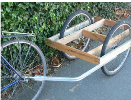
The completed trailer attached to the bike
