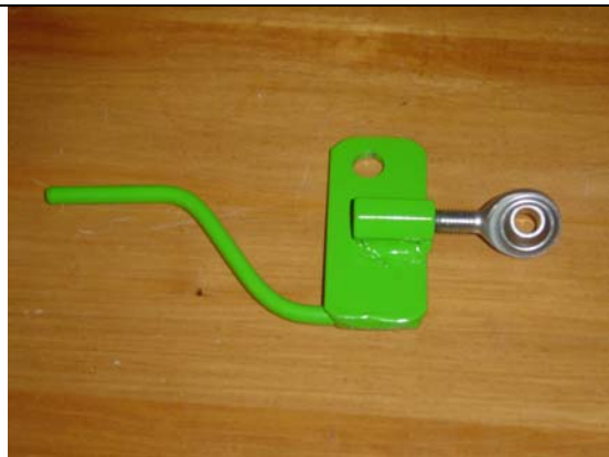
The hitch base bolts onto the rear axle and the rod end screws in.
