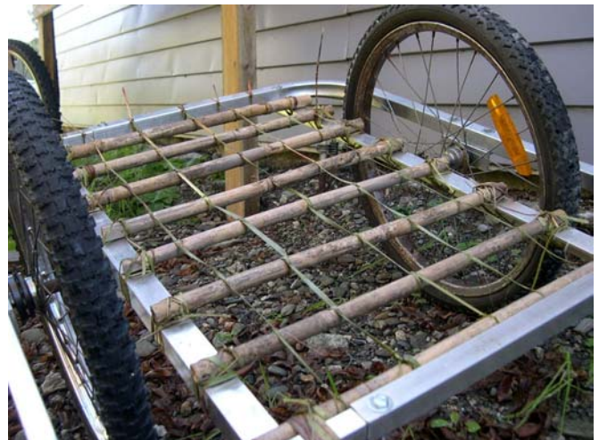
A novel light weight flax deck system fitted to one of the trailers.
